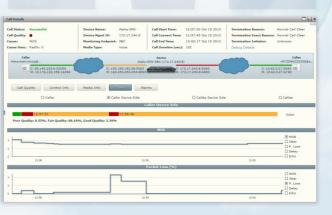
information, trends and alarms. Call trends enable rapid analysis of the call performance over the entire call duration, including time-based views of MOS, jitter, packet loss, delay and echo.
